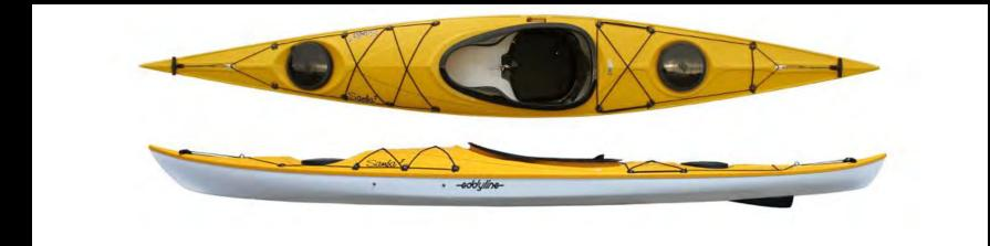
Length: 13' 10" | Beam: 22.5" | Weight: 43 lbs | Cockpit Size: keyhole 31.5" x 16.5" | Capacity: 300 lbs | Stability: Med
